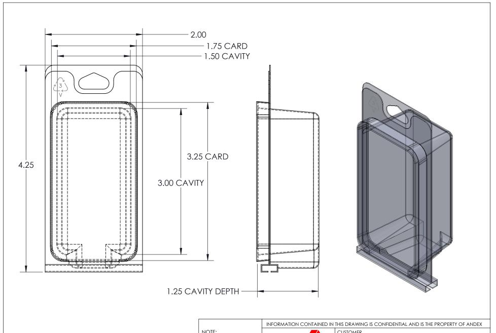
NOTE: ALL MATERIAL THICKNESS IS ± 10% PRIOR TO FORMING DRAFT ANGLES 5° TYP.
