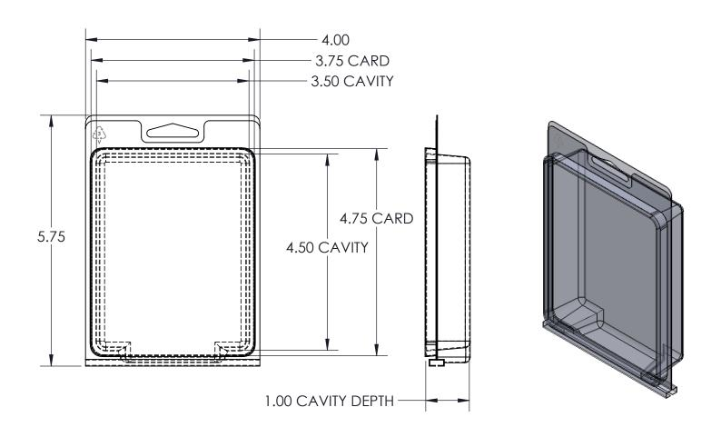
INFORMATION CONTAINED IN THIS DRAWING IS CONFIDENTIAL AND IS THE PROPERTY OF ANDEX NOTE: CUSTOMER ANDEX STOCK ALL MATERIAL THICKNESS IS ± 10% PRIOR TO FORMING **DESCRIPTION** 3122 ITEM NO. 1911 FOURTH AVE, NORTH ESCANABA, MI 49829 DRAFT ANGLES 5° TYP.
